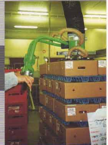
Palletising of cartons with extended handle
