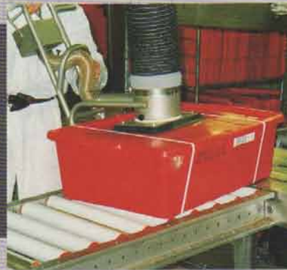
Handling of cases with extended articulated handle
